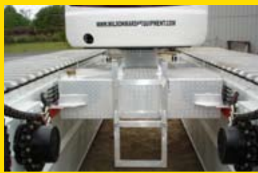
Auxilliary Fuel Tanks with Ladder
